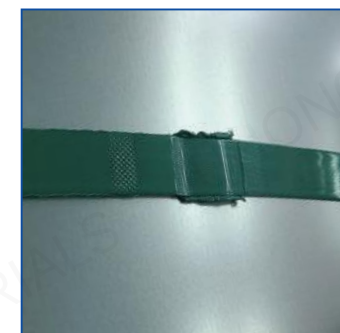
摩擦热熔 Friction-welded
