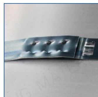
模切免扣连接 Die-cut sealless joints
