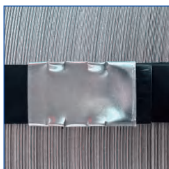
打包扣连接 Seal joint
