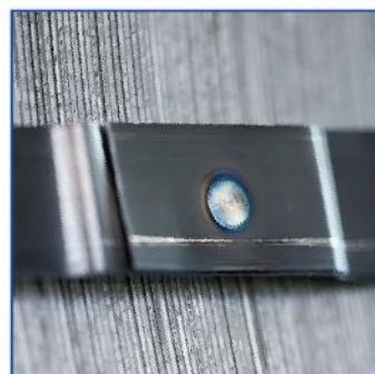
点焊免扣连接 Spot-weld sealless joints
